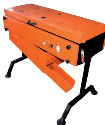
Fig. 3.4.11 Portable semi-automatic cashew apple and nut separator
