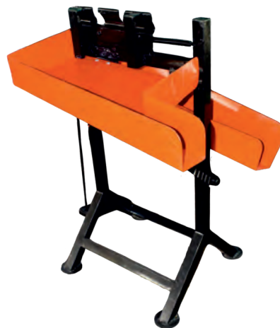
Fig. 3.4.10 Pedal-operated cashew apple and nut separator
