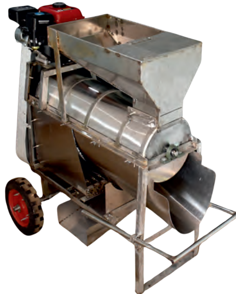
Fig. 3.4.12: 3-in-1 cashew nut separator, juice & pulp extractor, and fibrous material separator
